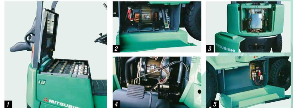
1. Battery 2. Hydraulic Motor 3. Controller 4. Traction Motor 5. Contactors
